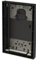
Flush-mounted box for mounting of outdoor station into the wall. This box is fitted with knock down holes for cabling from left, right, or back.
